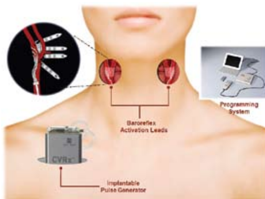
Diagrammatic representation of the baroreceptor stimulator system illustrating the implantable battery/pulse generator placed subcutaneously in the infraclavicular location, the electrode activation leads wrapped around the carotid bifurcation, and the computer-based programming system.
